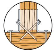
Double-shear nailing shall use full length common nails
